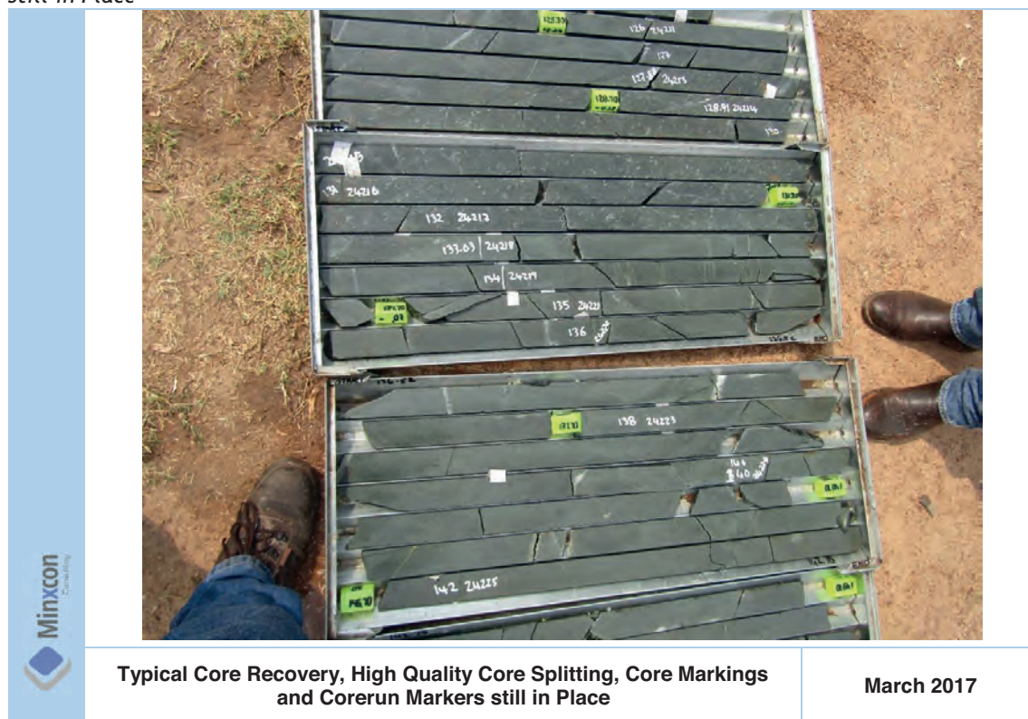
Figure 4: Typical Core Recovery, High Quality Core Splitting, Core Markings and Corerun Markers still in Place
