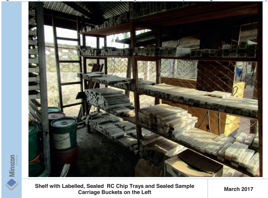
Figure 2: Shelf with Labelled, Sealed RC Chip Trays and Sealed Sample Carriage Buckets on the Left
