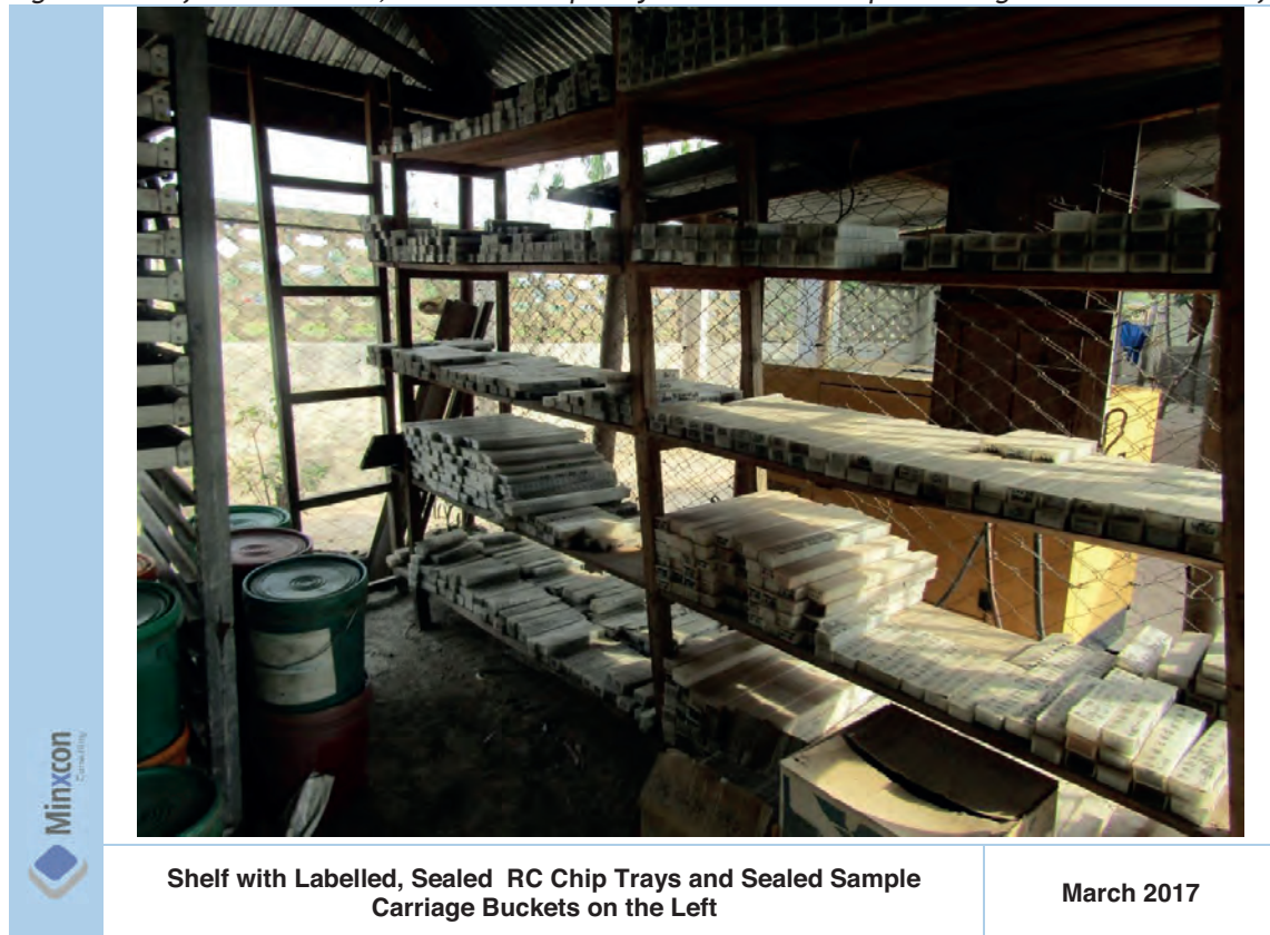
Figure 3: Shelf with Labelled, Sealed RC Chip Trays and Sealed Sample Carriage Buckets on the Left
